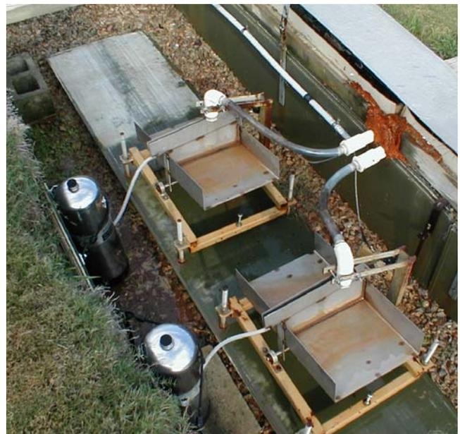
Detail of tipping bucket apparatus to measure runoff volume and take a sample in the slot between the two sides.
