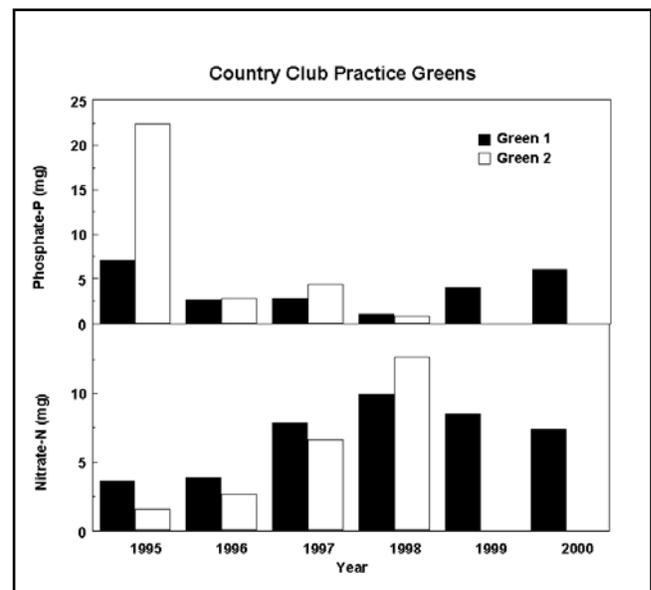
**Figure 1.** Phosphate and nitrate leached from two practice greens at a country club in Atlanta, GA, as the average of individual rainfall events for each year from 1995 to 2000. Greens were built in the fall of 1994, and Green 2 was removed in the winter of 1998-1999.
