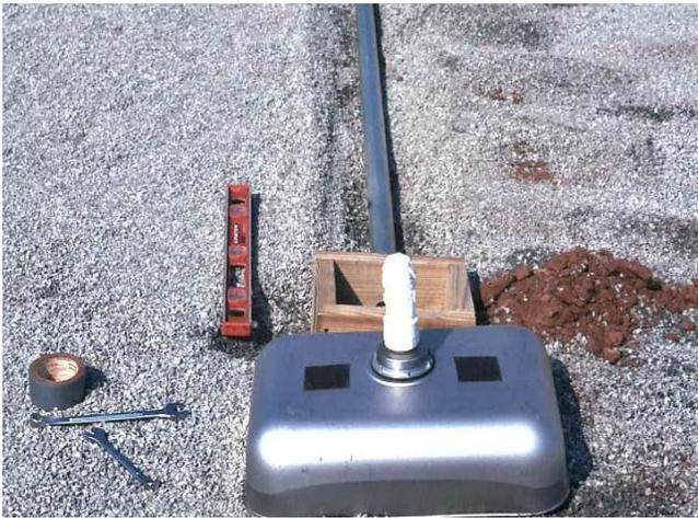
Lysimeters were constructed using stainless steel kitchen sinks (shown here inverted before installation) that collected the putting green leachate and allowed it to be collected in collection bottles at the edge of the greens.
