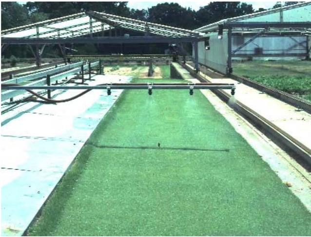
Field lysimeter facility to determine leaching of nitrate-N and phosphorus through simulated golf greens. There is a tunnel under the metal area to the left to sample leachate in bottles and a moving cover automatically cover the area during natural rainfall.
