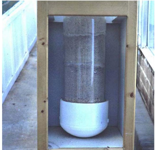
Column like those under turf boxes to simulate golf greens in the greenhouse to determine leaching of nitrate-N and phosphorus.
