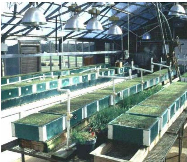
Simulated greens in a greenhouse to determine leaching of nitrate-N and phosphorus. The turf boxes shown have columns underneath built to U.S. Golf Association recommendations.
