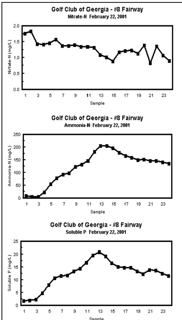
**Figure 6.** Concentrations of nitrate-N, ammonium-N, and phosphorus in runoff for a golf fairway in a northern suburb of Atlanta, GA. The samples are for one-hour intervals for a 1.5-inch rainfall event after applying ammonium phosphate to the fairway at a rate to give 1 lb. N/1000 sq. ft.
