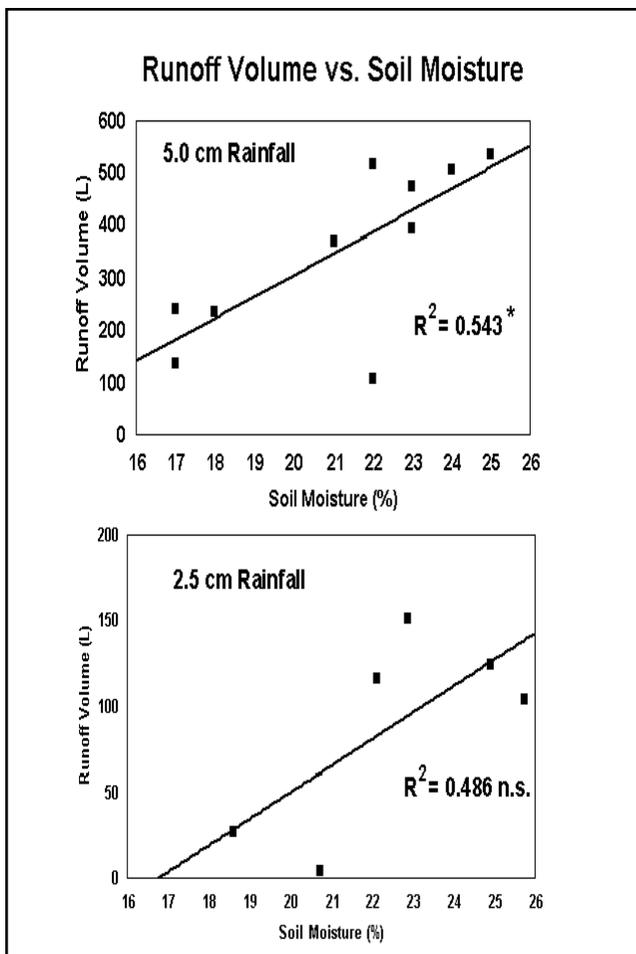
**Figure 7.** Runoff volume versus soil moisture before the simulated rainfall events. The runoff is for a field experimental site on a 5% slope to simulate a golf fairway.
