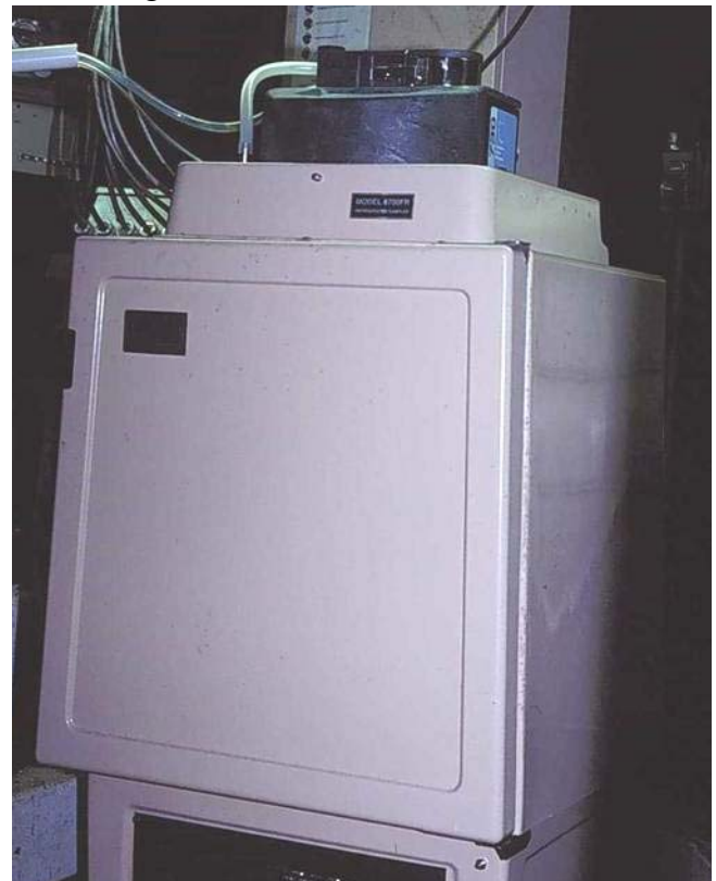
Figure 3. Leachate samples were taken every 30 minutes and stored within an automatic sampler.
