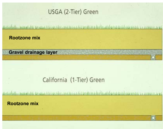
Figure 1. Cross-section diagrams of the soil profile for a one-tier and two-tier putting green.
