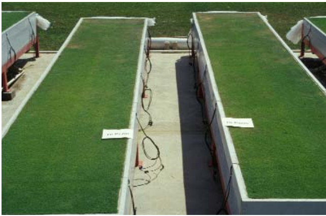
Figure 7. The higher permeability, one- and two-tier putting greens oriented to 4 % slope after 10 days without rain or irrigation. Turf in the foreground (downslope) does not show drought stress where turf in the background (upslope) does.
