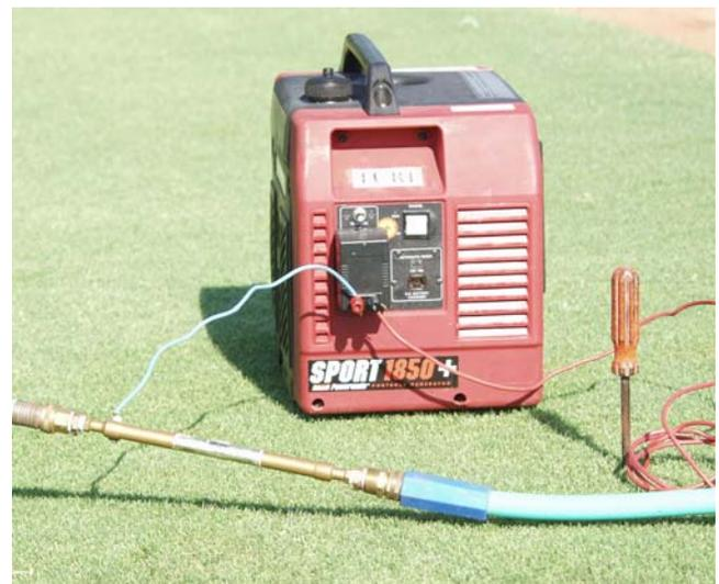
Figure 1. The Care Free Water Conditioner, classified as a catalytic water conditioning device, is shown hooked to irrigation hose and a DC voltage converter in an "active water treatment" setup.
