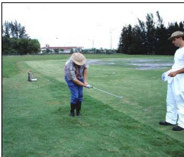
After Dr. John L. Cisar swung a golf club through grass treated with pesticide (center), an analysis was made of pesticides on the club head that were wiped off with damp cheesecloth by Mr. Raymond H. Snyder (right).
