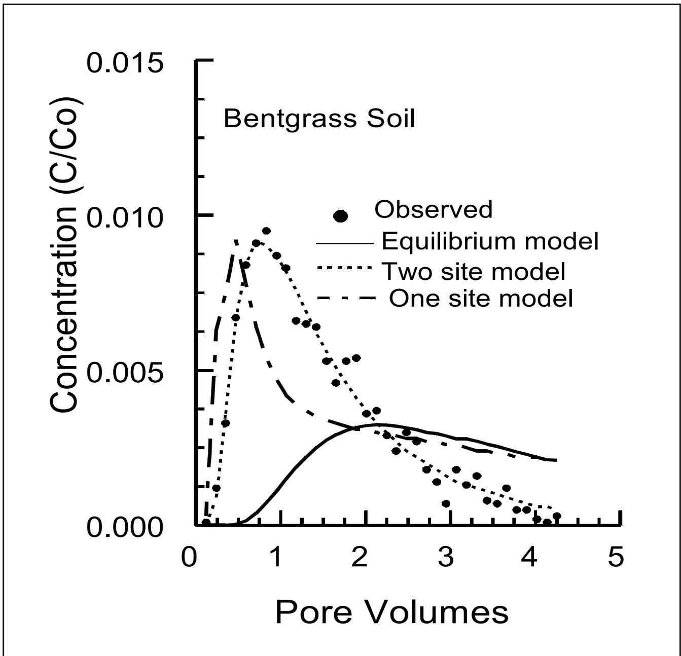
**Figure 2.** Breakthrough curves of 2,4-D applied to columns of bentgrass soil comparing observed versus an equilibrium model, and both one- and two-site non-equilibrium models. In pesticide breakthrough curves, the ratio of the relative concentration of pesticide exiting the soil column ( $C$ ) over the input concentration ( $C_0$ ) is calculated and plotted against the number of pore volumes that have exited the column.
