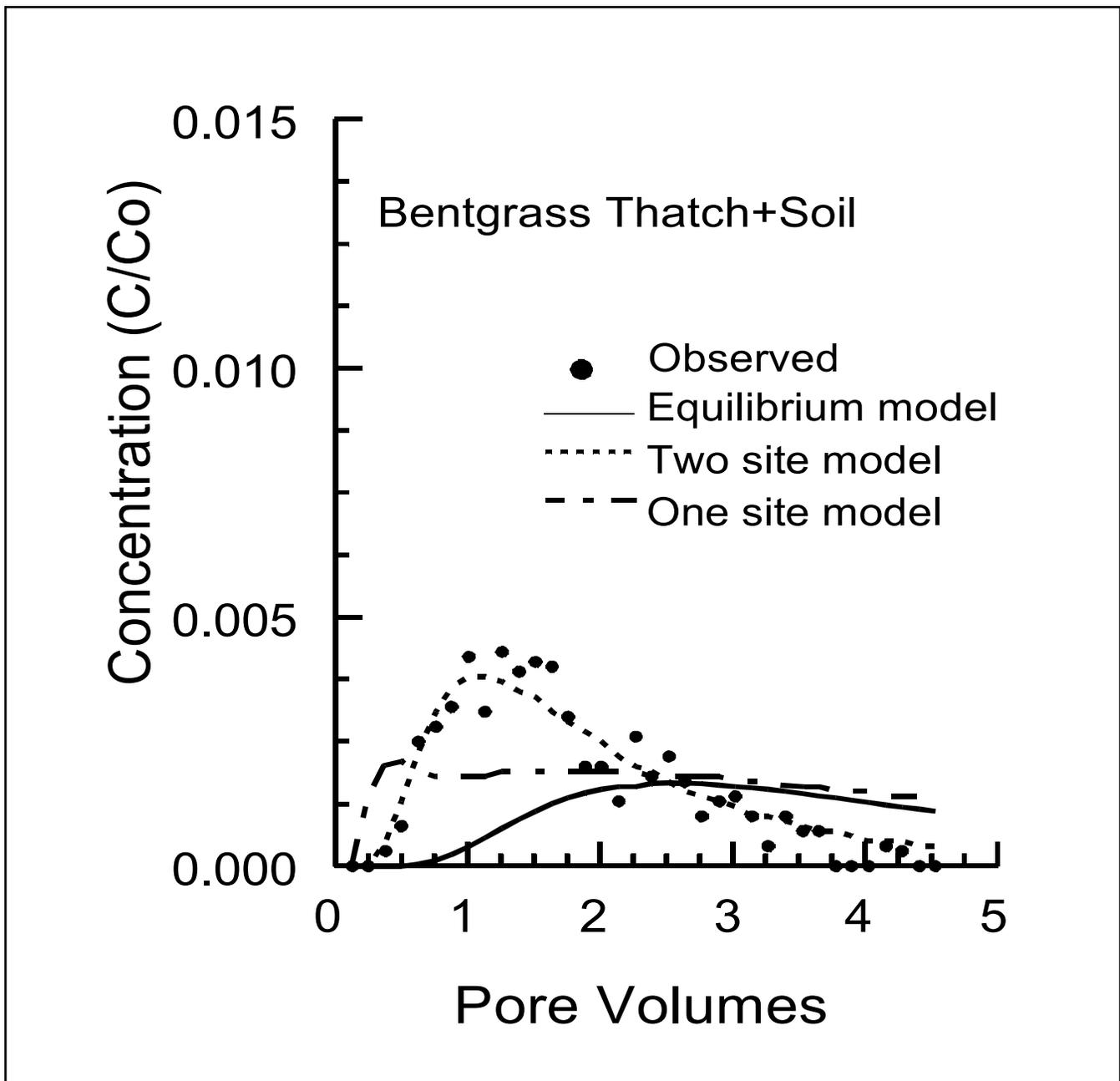
**Figure 3.** Breakthrough curves of 2,4-D applied to columns of soil and bentgrass thatch comparing observed, equilibrium model, and both one- and two-site non-equilibrium models. In pesticide breakthrough curves, the ratio of the relative concentration of pesticide exiting the soil column ( $C$ ) over the input concentration ( $C_0$ ) is calculated and plotted against the number of pore volumes that have exited the column.
